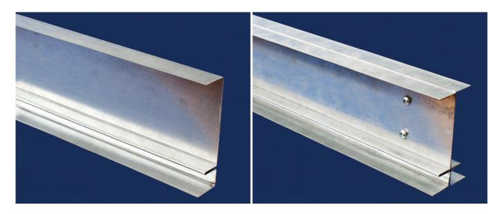
Protektor has developed a bespoke solution for shaftwall constructions, designed specifically for areas where a contractor cannot access both side of the partition. Our E profiles enable the contractor to construct the partition all from one side. The E profile holds the shaft side board in place without the need for screw fixings. The non shaft side boards are then attached with screws to the profile in the conventional manner.
