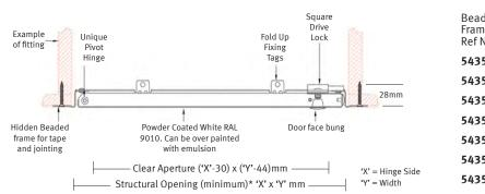
**Door Tray & Frame**: Formed from 1.0mm Zintec electro-galvanised mild steel with a 25mm wide frame either perforated or solid finished in polyester powder coat white RAL 9010 20% Gloss.
