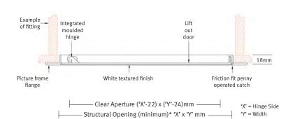
**Door Tray & Frame:** Moulded from UV stabilised ABS plastic with a 25mm wide picture frame to cover the cut edge of the aperture. Colour approximates to matt white RAL 9010 20% Gloss.
