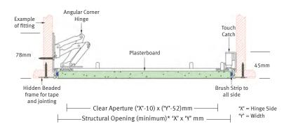
Door Tray & Frame: Formed from 1.0mm and Availability: Standard stock sizes available 1.2mm Zintec electrogalvanised mild steel 24 - 48 hours with Bespoke panels available with a 25mm wide perforated frame finished on request in ppolyester powder coat white RAL 9010
