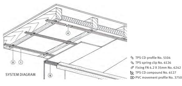
The joists should be no greater than 700mm apart and the TPS - CD Profiles should be fixed to the joist line. The profiles are then connected to the clip by "offering up" the channel and applying pressure. The CD Profile will lock in to the Spring Clip.
