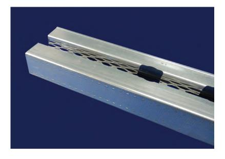
The Protektor Acoustic Stud profiles are manufactured for areas where a higher level of acoustic performance is required in a single non load bearing stud partition construction. Manufactured from 0.6mm Galvanised Steel the
