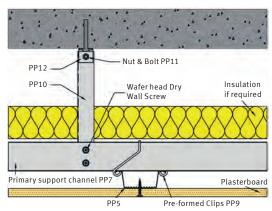
NOTE: Self-drilling dry wall pan head screws to be used in Domestic/ Residential Applications
