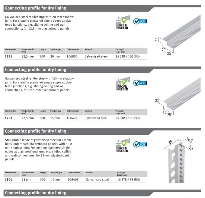
Stop profile made of galvanised steel for assemblies underneath plasterboard panels, with a 20mm shadow joint. For creating plastered single edges at plastered junctions, e.g. sliding ceiling and wall connections, for 12,5-mm plasterboard panels.
